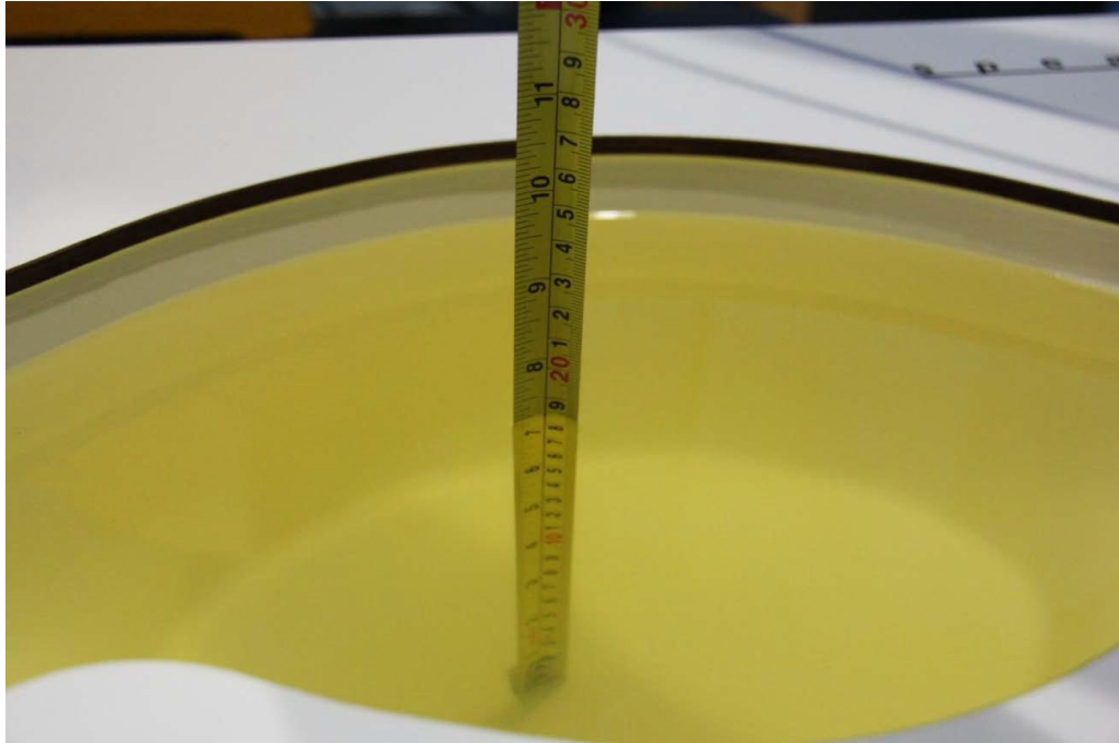
Picture 7-1: Liquid depth in the Flat Phantom(2450MHz)
