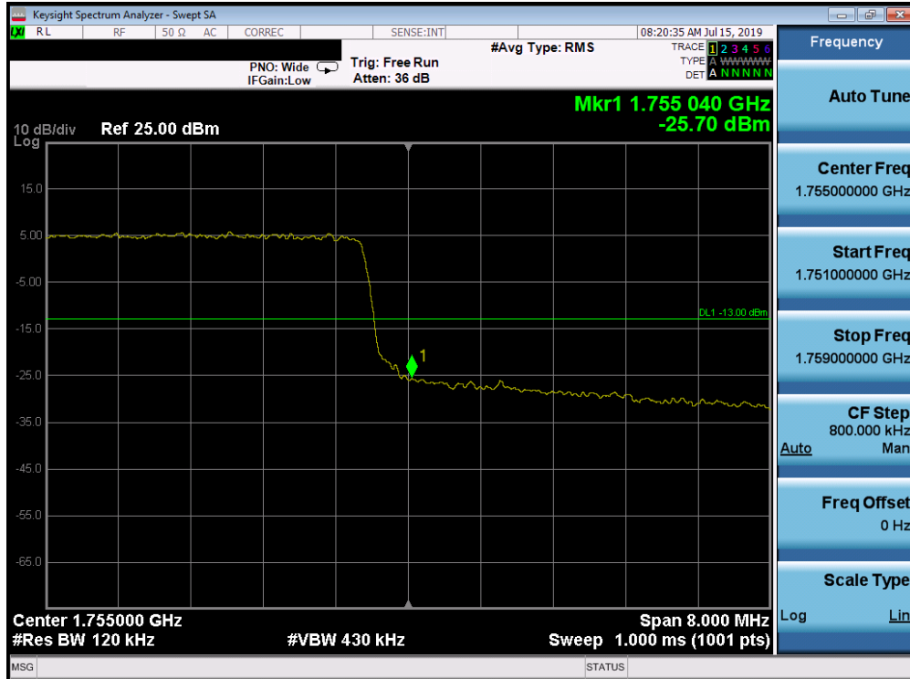
Plot 7-218. Upper Band Edge Plot (Band 4 - 10.0MHz QPSK - Full RB Configuration)
