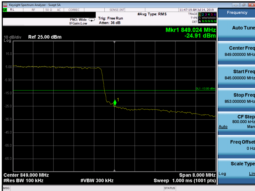
Plot 7-195. Upper Band Edge Plot (Band 26/5 - 10.0MHz QPSK - Full RB Configuration)
