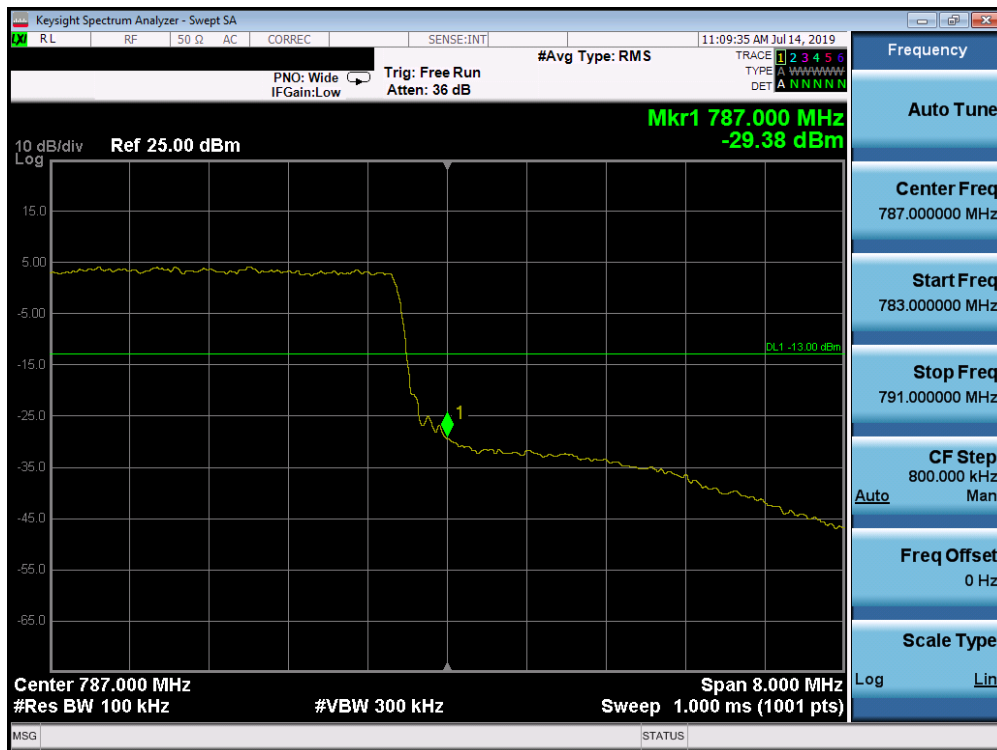
Plot 7-185. Upper Band Edge Plot (Band 13 - 10.0MHz QPSK - Full RB Configuration)
