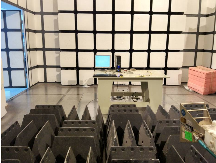
Radiated Emissions – Front View (Above 1 GHz)
