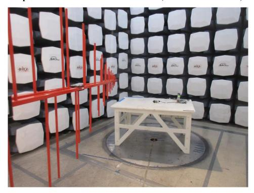
1.2 Radiated Spurious Emissions measured at 3 meters, 30 MHz to 1000 MHz, Rear View
