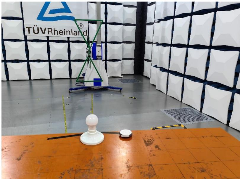
**Photograph 3: Set-up for measurement of radiated emission (1-18Ghz)**
