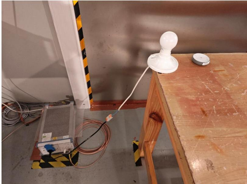
**Photograph 2: Set-up for measurement of radiated emission (30-1000Mhz)**
