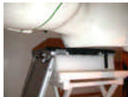
Figure 14.6.1 Body SAR Test Setup -- Laptop Vertical Position --
