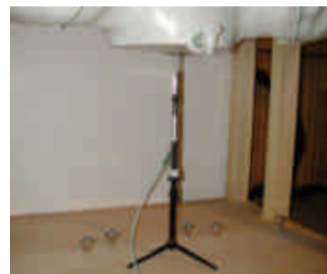
Figure 12.1 Dipole Validation Test Setup
