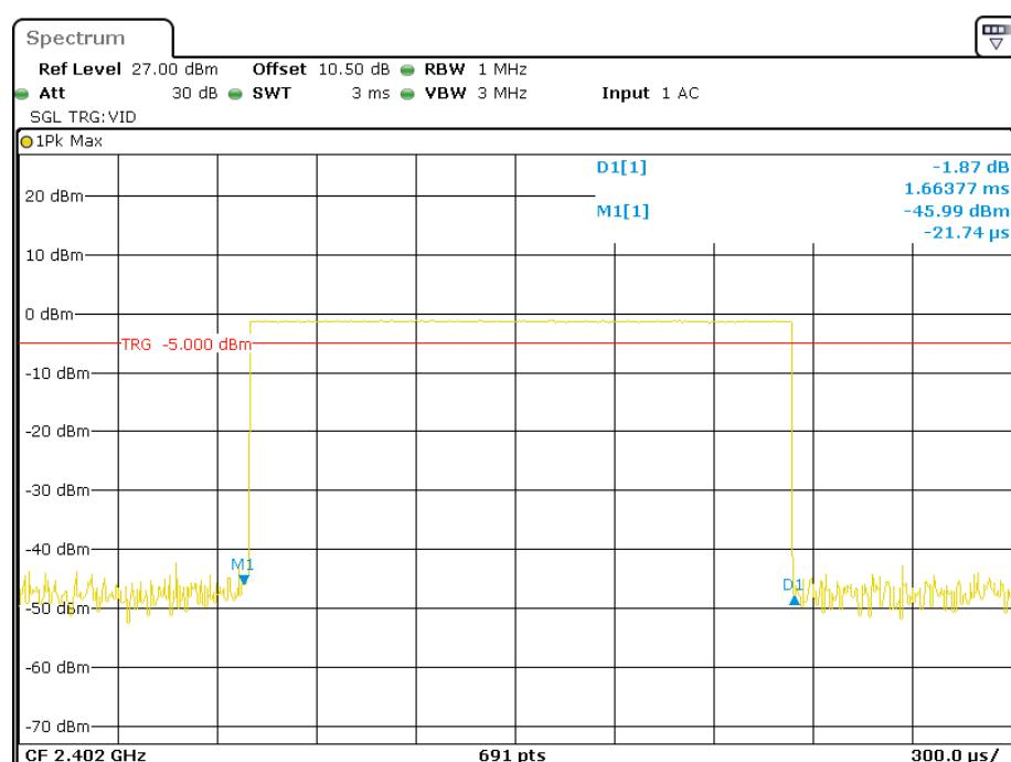
**Pulse time, Middle Channel, DH3**
