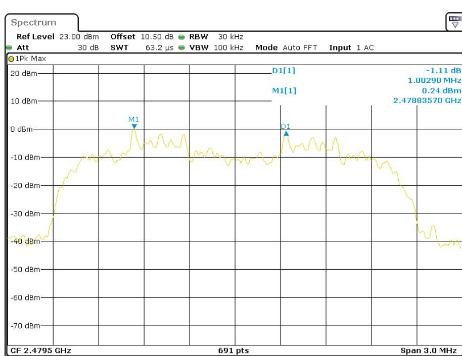
**EDR (8DPSK): Low Channel**
