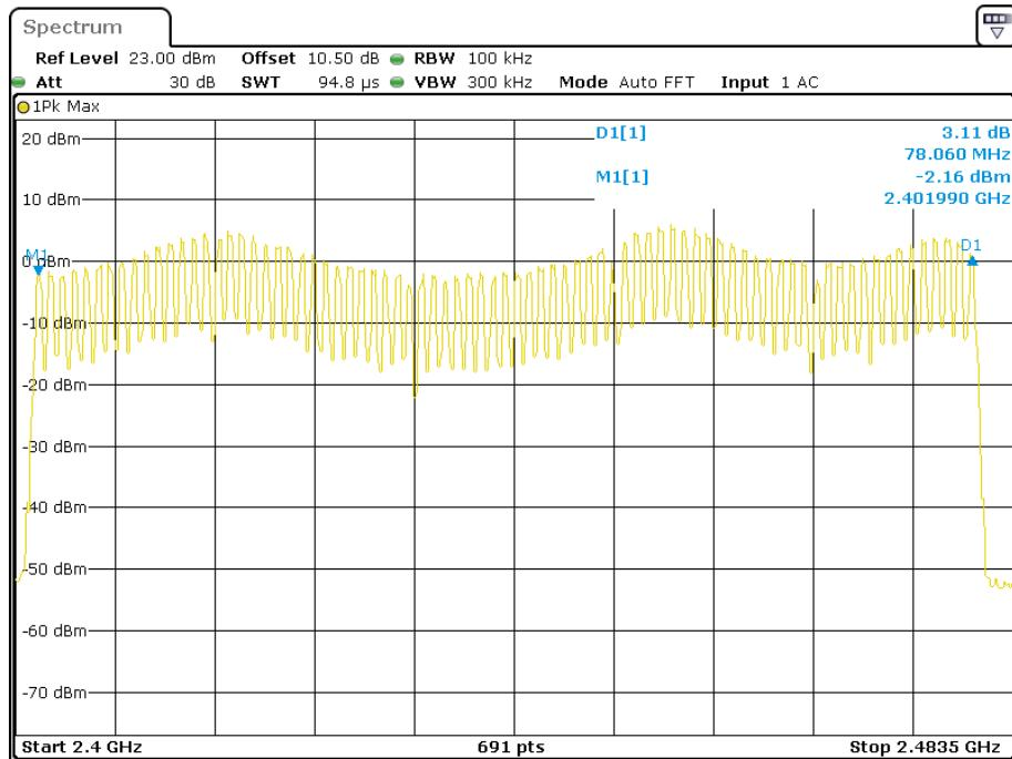
**EDR ( $\pi/4$ -DQPSK): Number of Hopping Channels**
