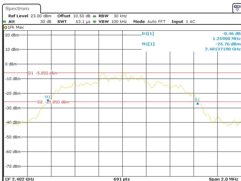
**EDR (8DPSK): Middle Channel**
