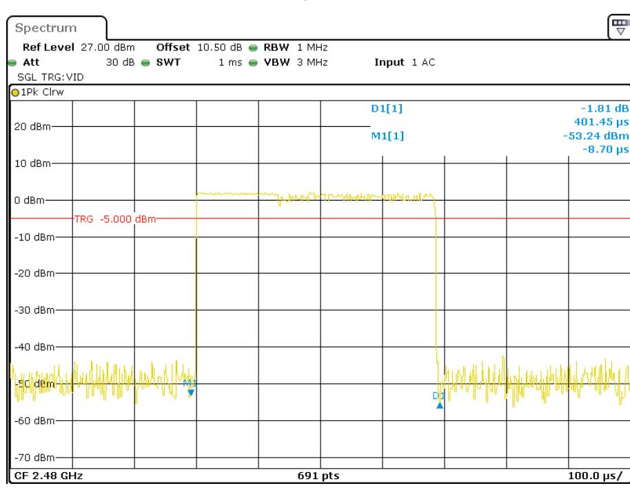
**Pulse time, Low Channel, 2DH3**
