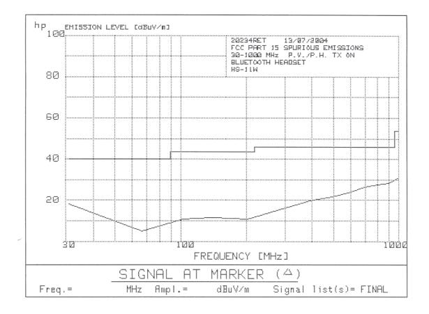
Resolution bandwidth = 100 kHz. Video bandwidth = 100 kHz. (This plot is valid for all three channels).
