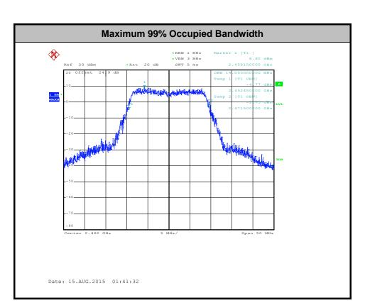
Note: The occupied channel bandwidth is maintained within the band of operation for all of the modulations.
