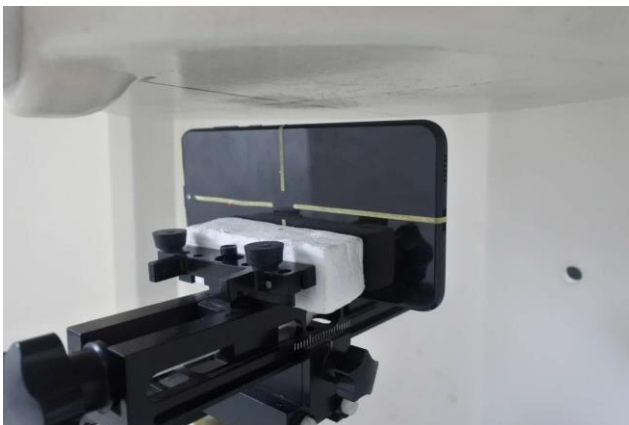
Right Side, Test Separation 10 mm
