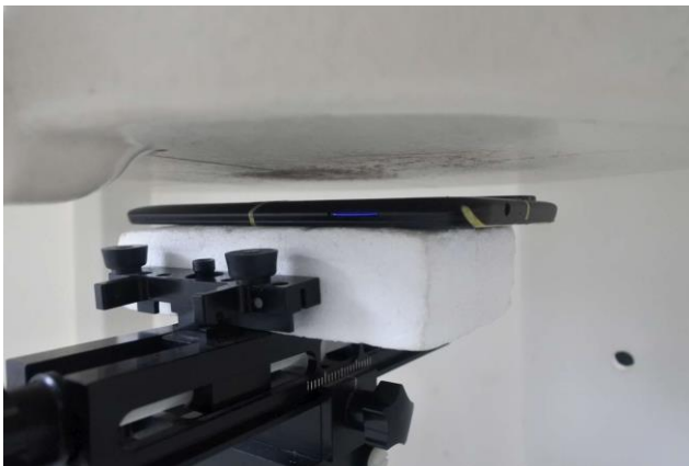
Back, Test Separation 10 mm
