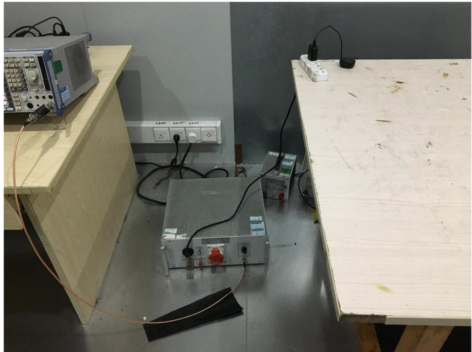
Conducted Emission Test Setup
