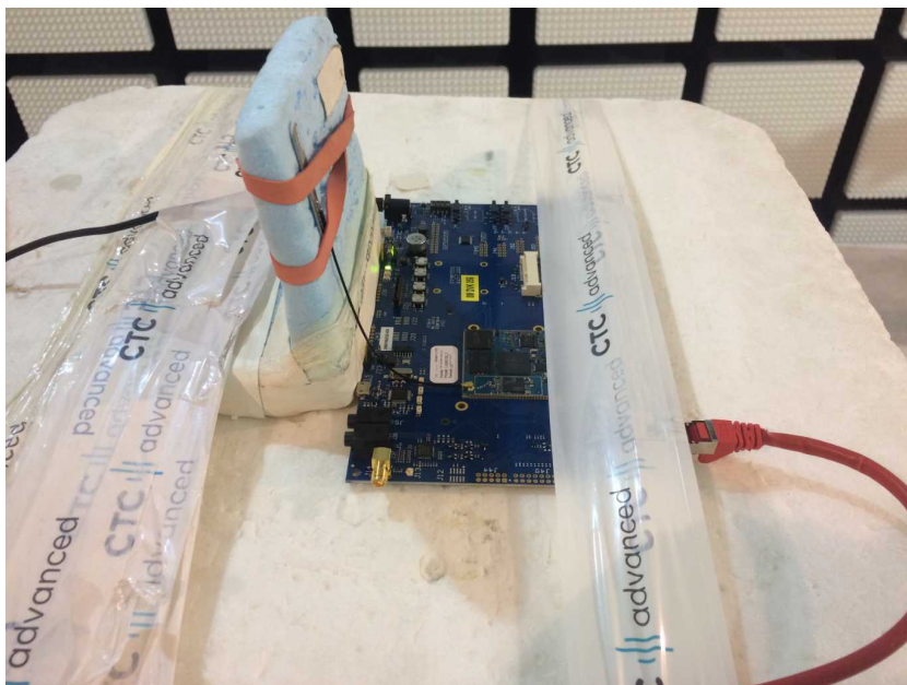
Photo 16: Fully anechoic chamber test setup (PCB Antenna, YAGEO ANT100P001B24553)
