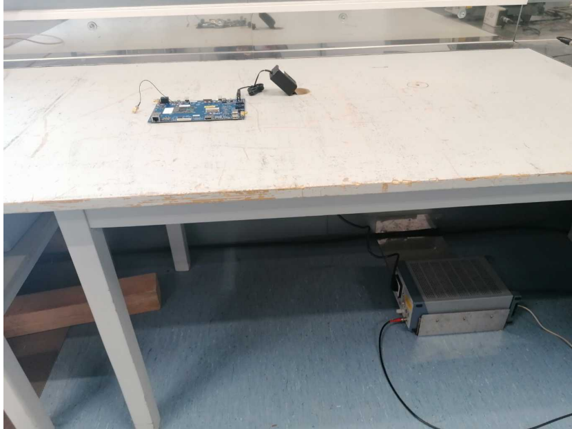
Photo 25 - Conducted AC Emissions (RF ports terminated)
