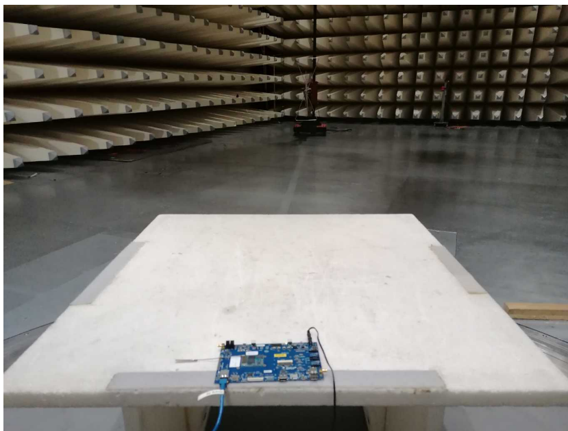
Photo 12: Semi anechoic chamber test setup (PCB Antenna, TAOGLAS FXP831.07.0100C)
