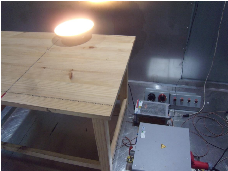
Photograph 2: Set-up for measurement of radiated emission
