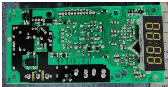
Note : New mother board is the same of circuit function with original. They have the same input/output rating and power are identical to the original. Only some electronic components and PCB layout differences.
