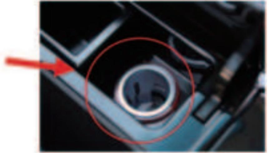
Note: Please use the standard car cigarette lighter. If you do not use our original power adapter, you need to buy a high-quality power adapter that meets the standard. Otherwise, due to insufficient voltage and current and excessive heat, it is easy to damage the smart screen or cause other damage, and the frequency modulation (FM) transmission function will not work properly.
