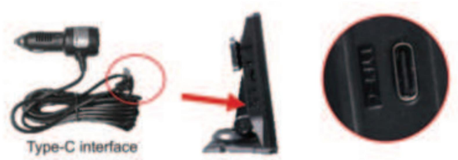
3: Insert the power adapter into the vehicle cigarette lighter socket, and sort out the power harness.
