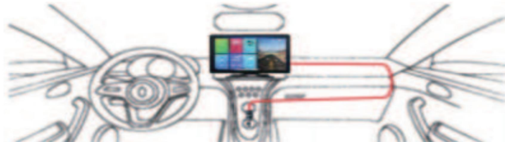
5: Turn on the recording function of the driving recorder, adjust the camera Angle to ensure the recording direction, and then tear off the 3M glue at the bottom of the bracket and fix the smart screen on the center console.
