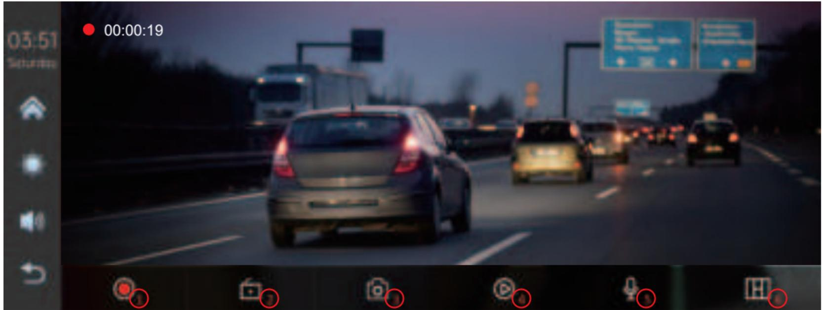
1: Record switch, 2: lock record switch, 3: take pictures, 4: playback, 5: record switch, 6: current video selection
