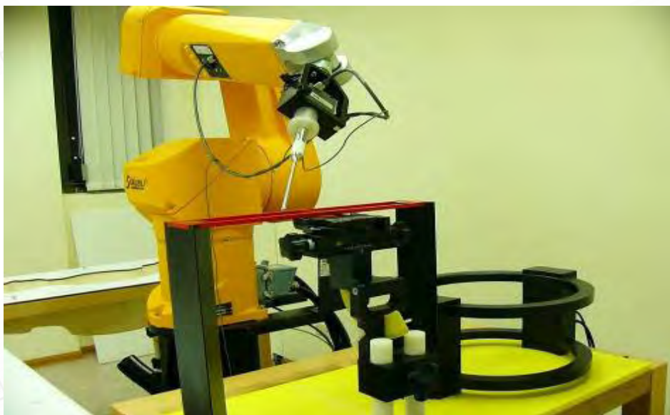
Fig. 1 Photograph of the DASY 5 measurement system
