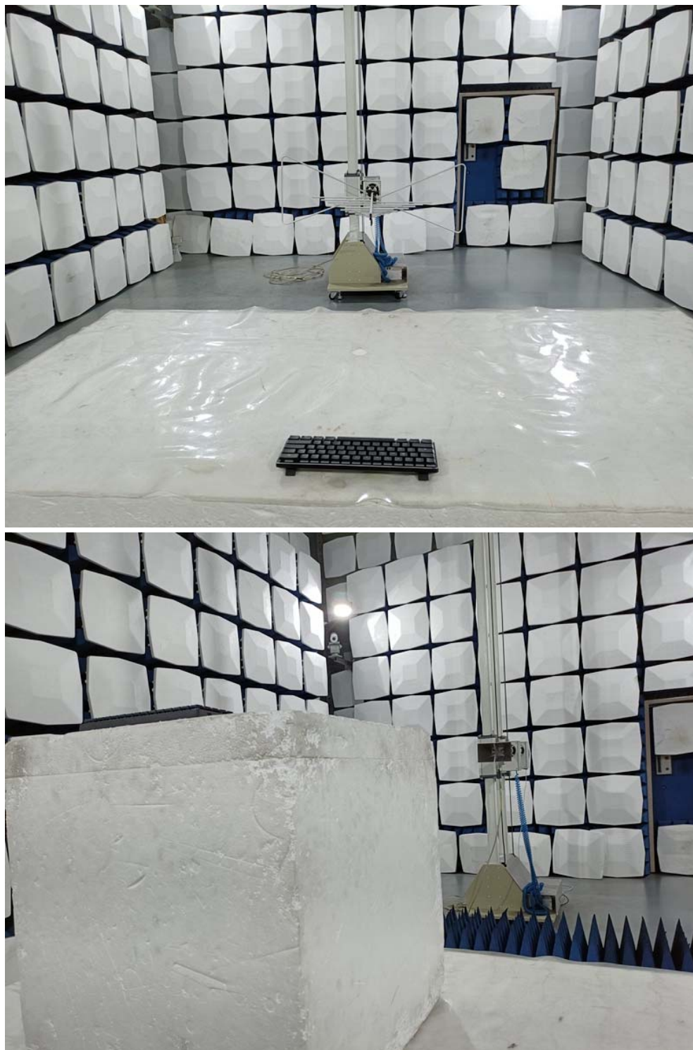
Radiated emission test view
