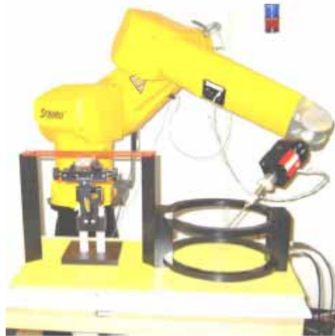
Figure 5.4-1: T-Coil set up with HAC Test Arch with Helmholtz Coil (AMCC)
