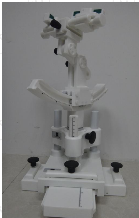
COMOSAR Mobile phone positioning system
