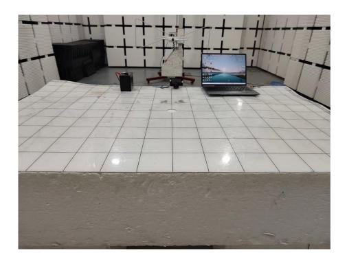
Set-up for Radiated Spurious Emission, Above 1GHz
