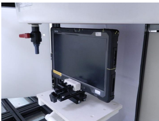
Edge1, Test Separation 15 mm
