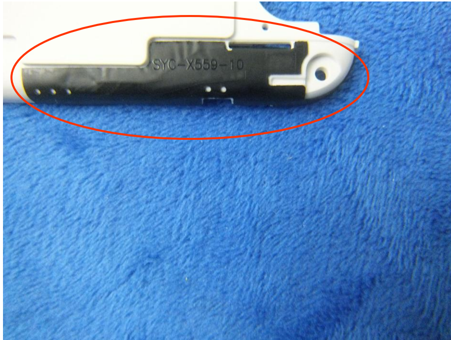
GSM/PCS/UMTS - Antenna View
