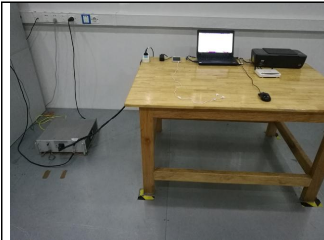
Conducted Emissions Test Setup – Front View
