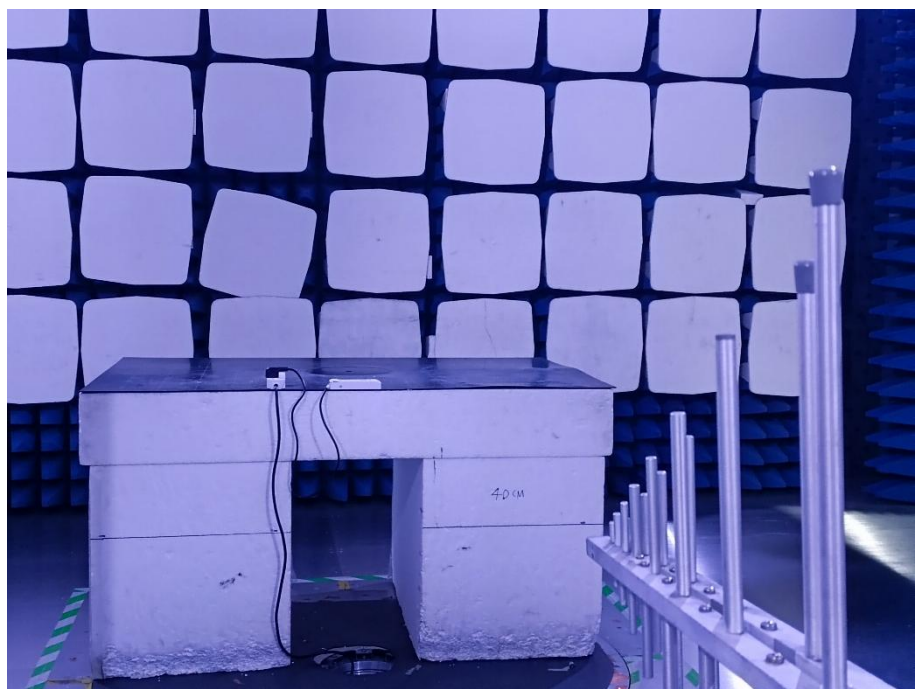
Radiation Emission Test Setup (30MHz to 1GHz)
