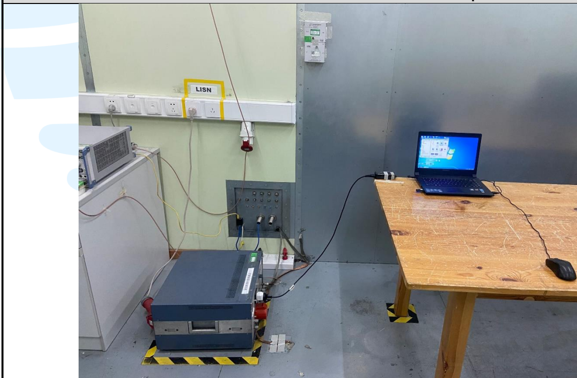
AC Power Line Conducted Emission Test Setup
