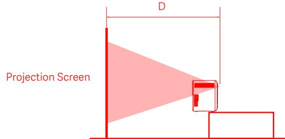
Determine the distance between the projector and the screen according to the desired screen size.
