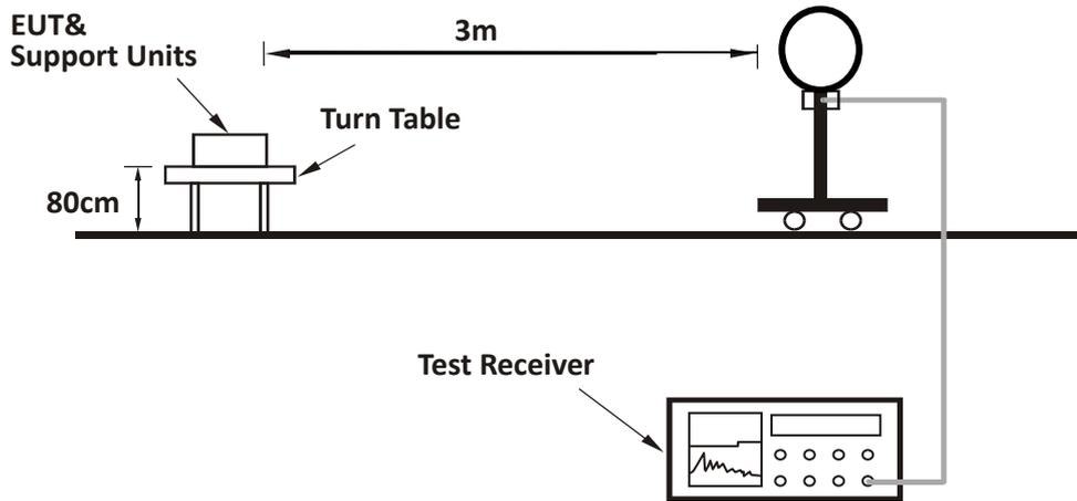
**For Radiated emission 30MHz to 1GHz:**
