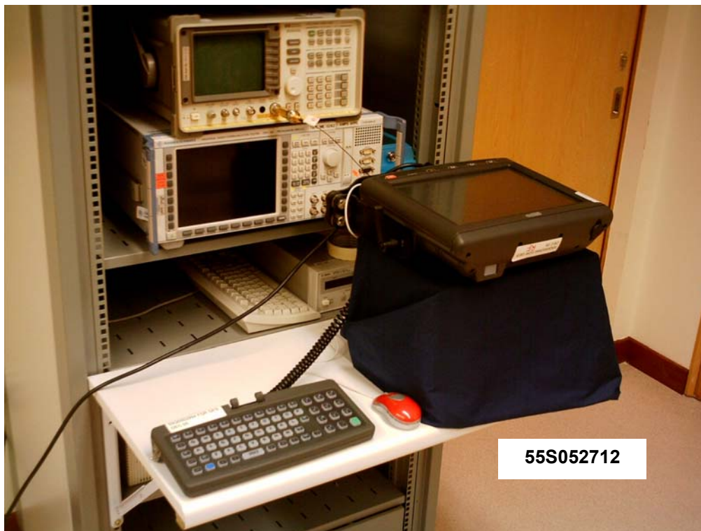
Spectrum Bandwidth (20dB Bandwidth Measurement) Test Setup
