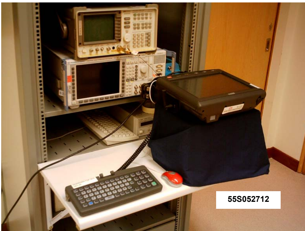
RF Conducted Spurious Emissions Test Setup
