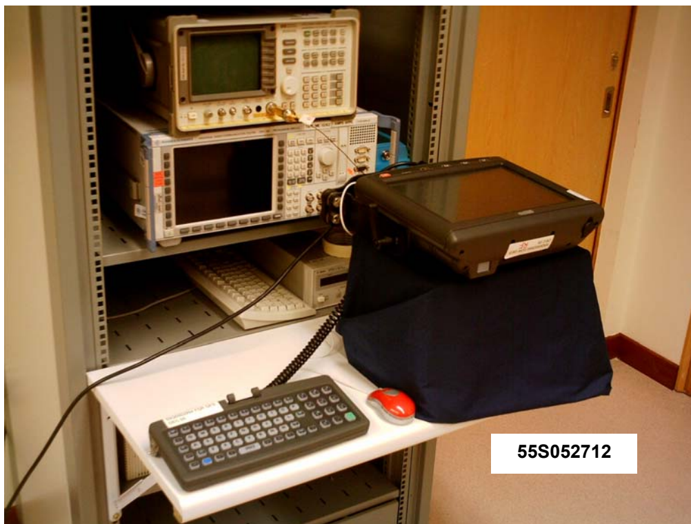
Peak Power Spectral Density Test Setup
