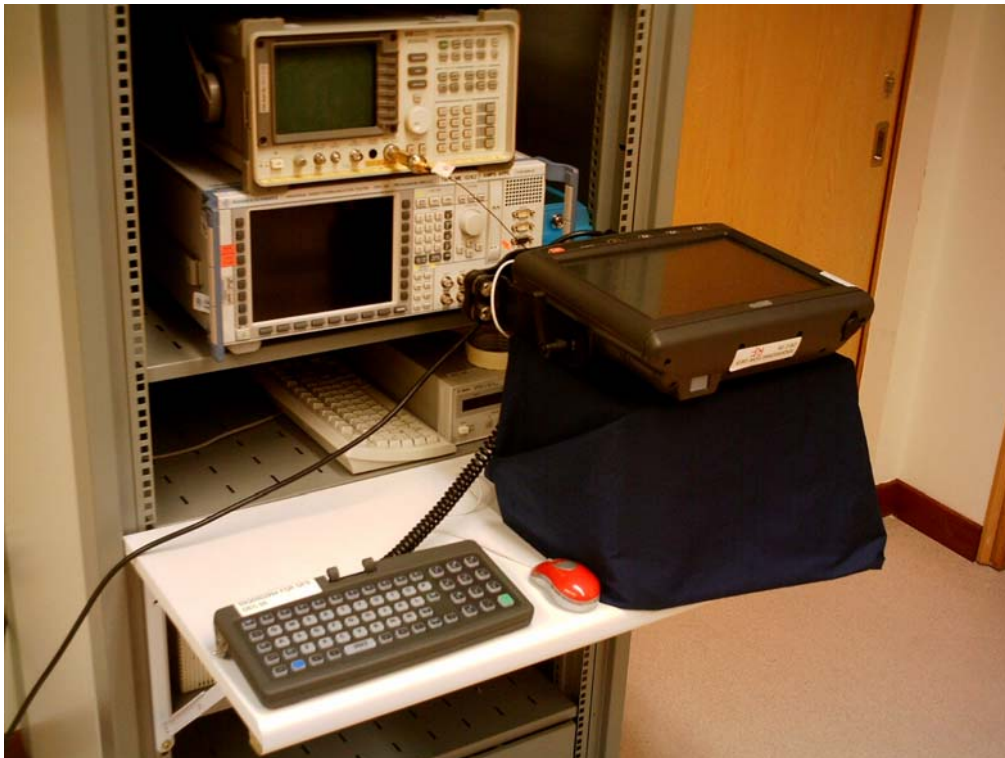
Maximum Output Power Test Setup
