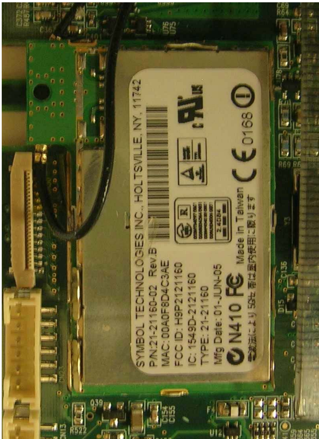
WLAN (802.11a/b/g) Module (With RF Shield)
