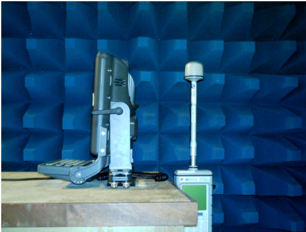
Maximum Permissible Exposure (MPE) Test Setup
