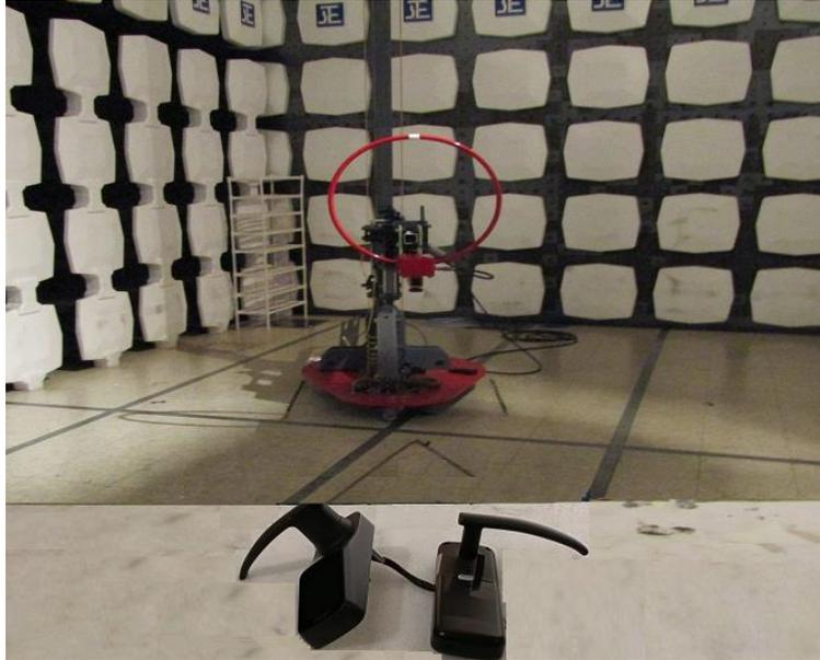
**Measurement of Radiated Emission Test Set Up**
