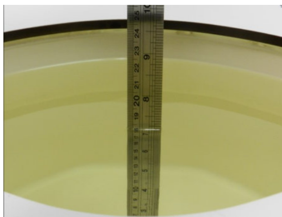
Fig 11.2 Photo of Liquid Height for Body SAR
