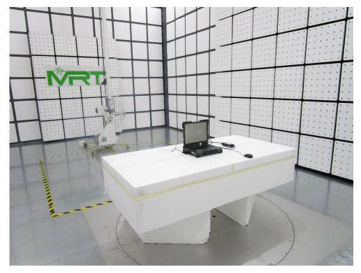
Description: Radiated Emission Test Setup for 1~18GHz
