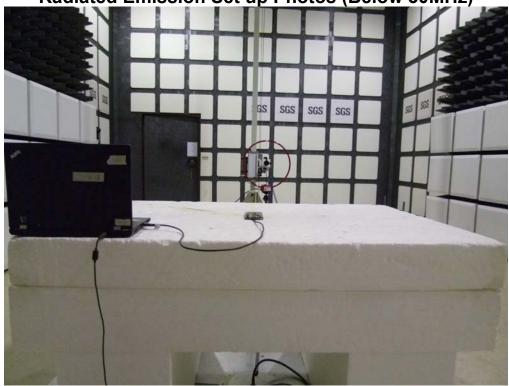
Radiated Emission Set up Photos (Below 1GHz)
