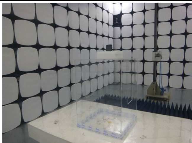
Radiated Spurious Emissions Test Setup Above 1GHz
