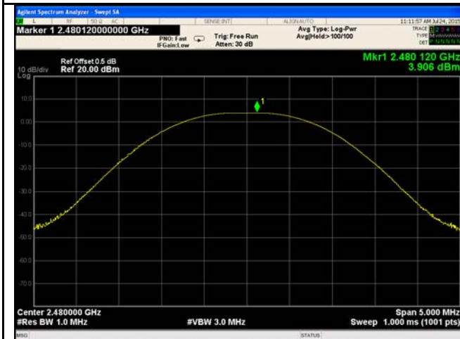
GFSK Output power - High CH 2480
