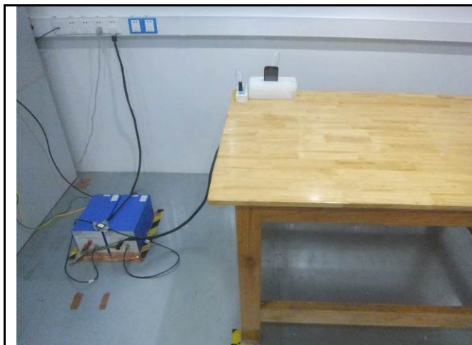
Conducted Emissions Test Setup Front View
