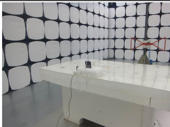
Conducted Emissions Test Setup Front View
