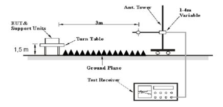
The radiated emission tests were performed in the 3 meters test site, using the setup accordance with the ANSI C63.10-2013. The specification used was the FCC 15 § 15.209, 15.205 and 15.231.
