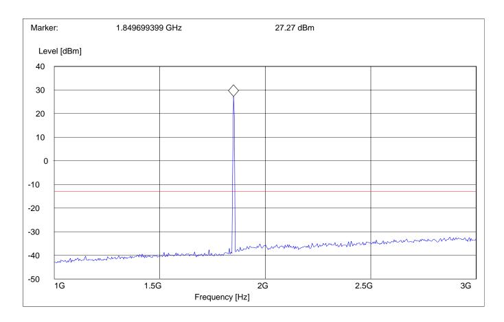
RADIATED SPURIOUS EMISSIONS Tx @ 1850.2MHz: 3GHz – 18GHz
