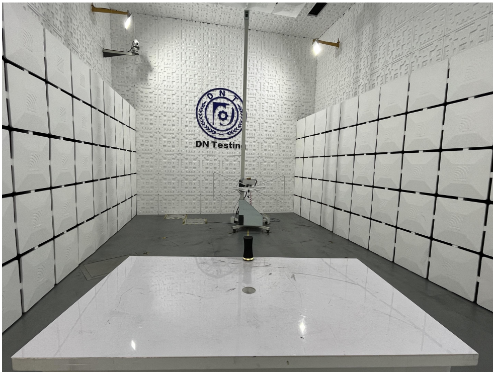
Radiated Emission Test View|(Below 1G)
