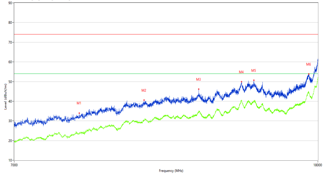
REmission Test case_FCC_Part 15C_FCC 15.247_7GHz-18GHz
