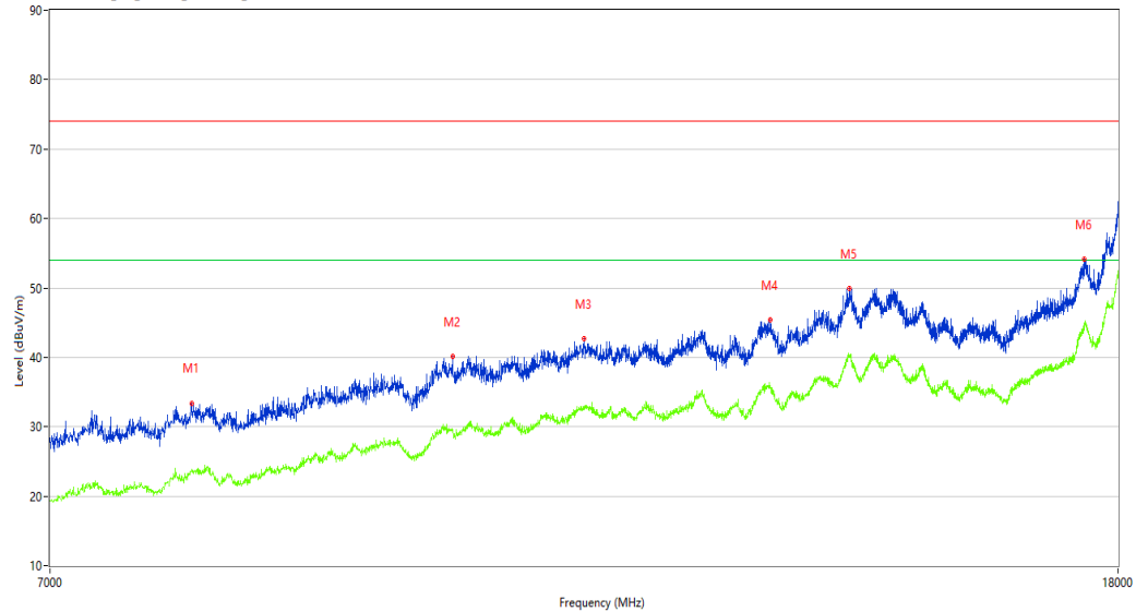
REmission Test case_FCC_Part 15C_FCC 15.247_7GHz-18GHz
