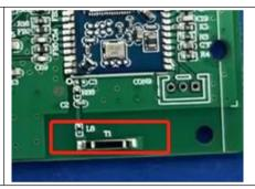
The antenna is Chip antenna.
