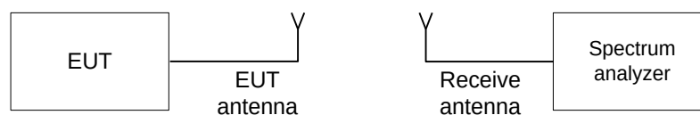
Figure 7.1.1 The 20 dB bandwidth test setup
