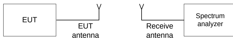
Figure 7.2.1 Carrier frequency separation test setup
