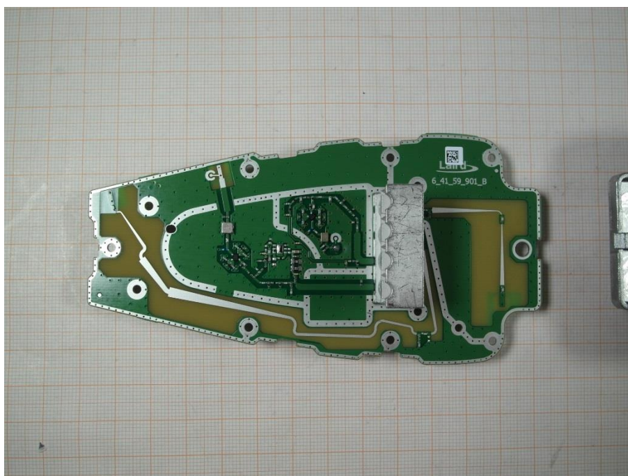
Photo 12: Antenna bottom site with connector and matching networks
