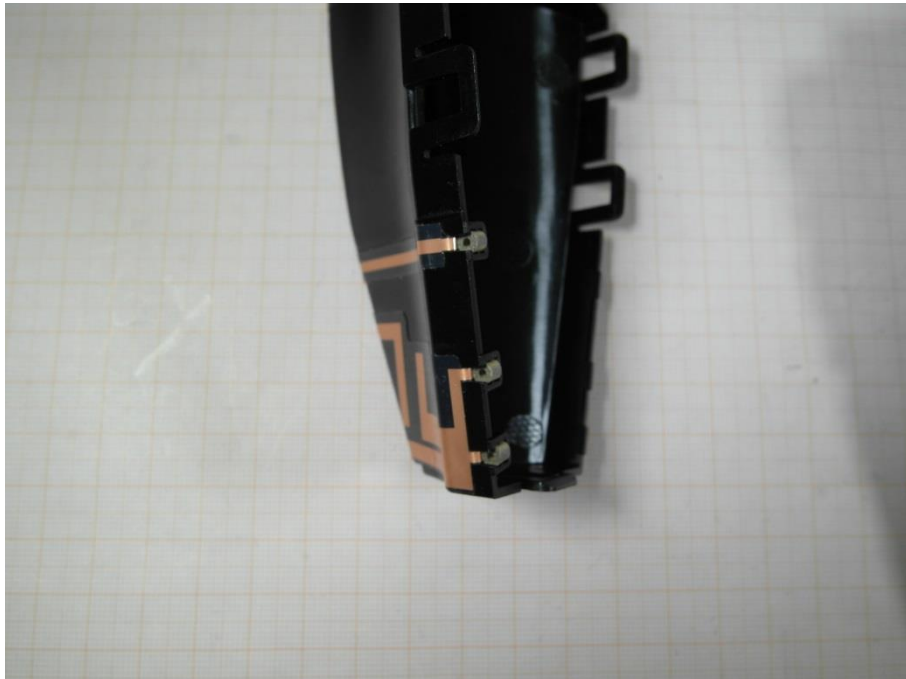
Photo 10: Foil antennas with connectors
