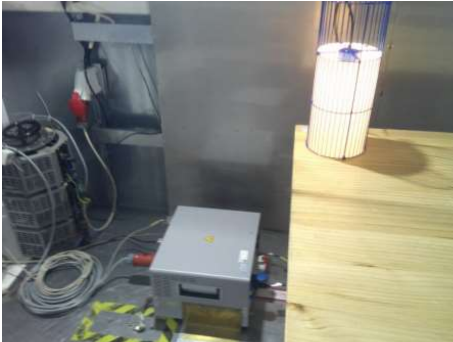
Photograph 1: Set-up for measurement of conducted emission
