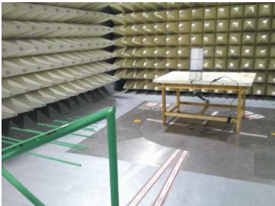
Photograph 2: Set-up for measurement of radiated emission
