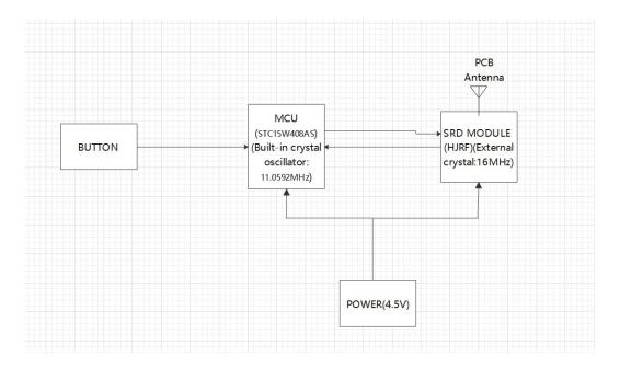
The module is welded on the PCB of end product, and the new added host are HJSR79, HJSR79B and HJSR79C. The hosts are all remote controllers, the hosts function and description please refer to section 8, 9 and 10 of the manual.
