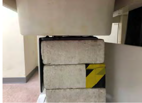
Fig.3 EUT Bottom side to flat phantom
