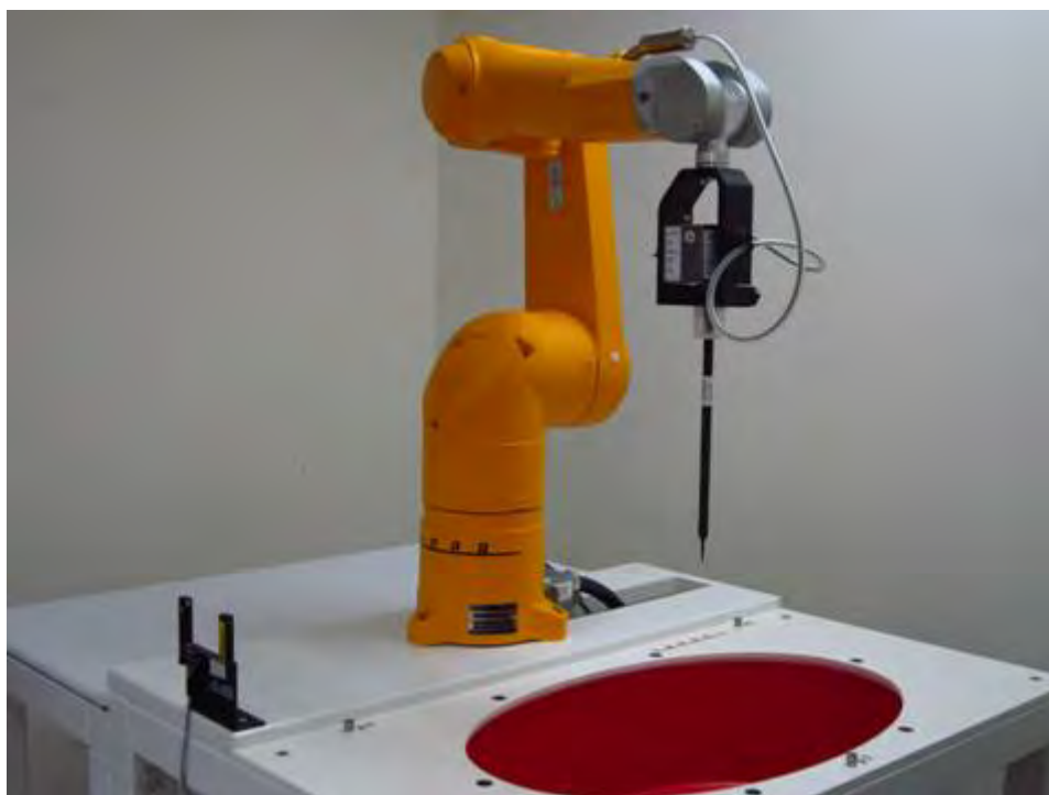
Fig.1 Photograph of the SAR measurement system
