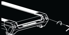
OVER TIME THE RUNNING BELT WILL LOOSEN. TO TIGHTEN THE BELT TURN THE LEFT & RIGHT SIDE BOLTS ONE FULL TURN CLOCKWISE. CHECK THE TENSION OF THE BELT, CONTINUE PROCESS UNTIL BELT IS THE CORRECT TENSION. ENSURE TO ADJUST BOTH SIDES EQUALLY TO CORRECT BELT ALIGNMENT.
