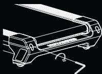
IF THE RUNNING BELT MOVES TO THE LEFT, TURN THE BOLTS ON THE LEFT SIDE  $\frac{1}{4}$  TURN CLOCKWISE, THEN TURN THE RIGHT BOLT  $\frac{1}{4}$  TURN COUNTER-CLOCKWISE. IF THE BELT DOES NOT MOVE, REPEAT UNTIL IT CENTRES.
