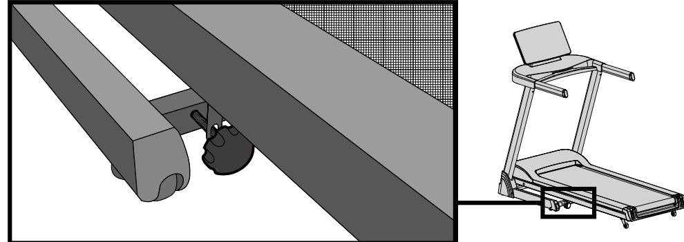
**(EN)** If you have to move the Treadmill whilst the running deck is down, ensure the locking pin is tightly in place, dismantle the Treadmill so the running deck and uprights are separate, then move the parts into place using two people and re-assemble. Remove the locking pin before use, failure to do so will prevent the incline from working and will damage the incline motor.
