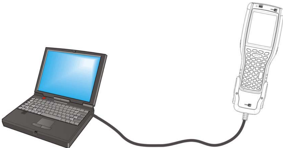
Figure 10: Direct Data Communication Using Snap-on Cable
