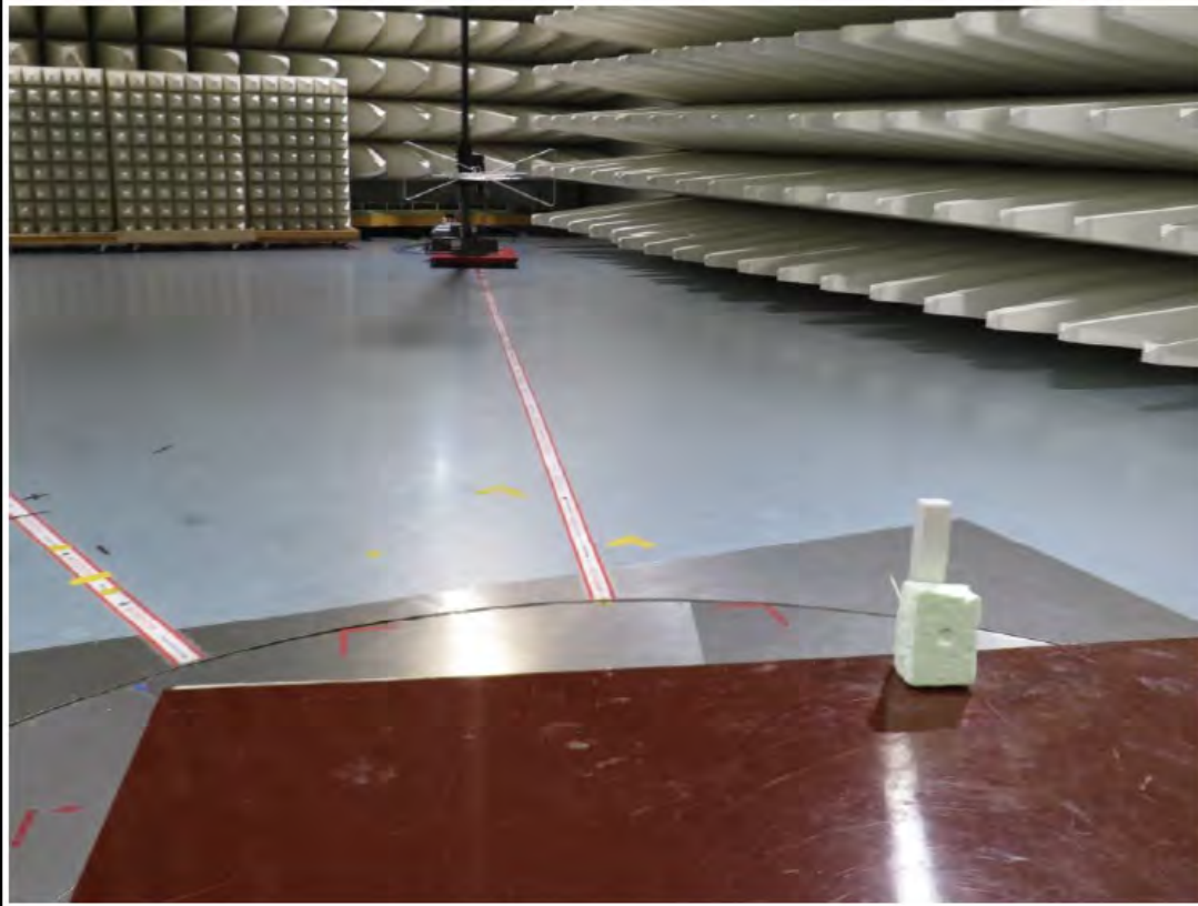
Test setup configuration 2 antenna VULB 9162 horizontal AC 6
