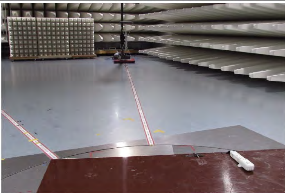
Test setup configuration 4 antenna VULB 9126 vertical AC 6
