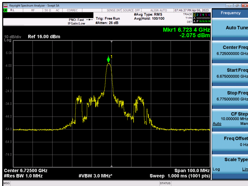
Plot 7-106. Power Spectral Density Plot MIMO ANT2 (40MHz BW 802.11ax (26 Tones) (UNII Band 7) – Ch. 155)
