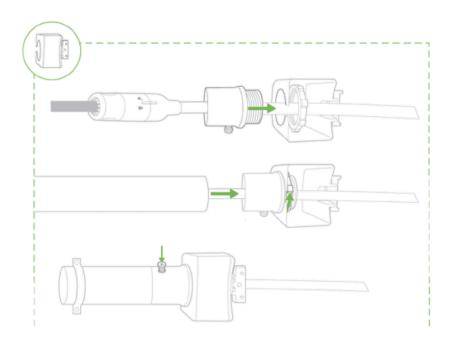
Installing the conduit box to MV73 series: (optional)
