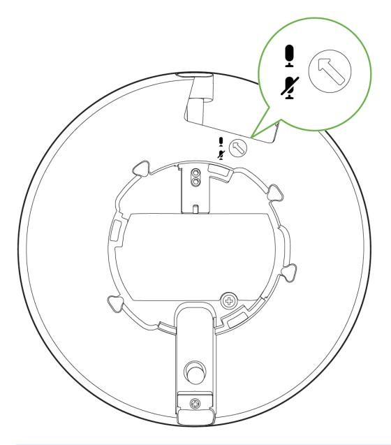
Note: If the microphone switch is disabled and the camera is mounted, toggling the switch back ON would require accessing the camera's base.
