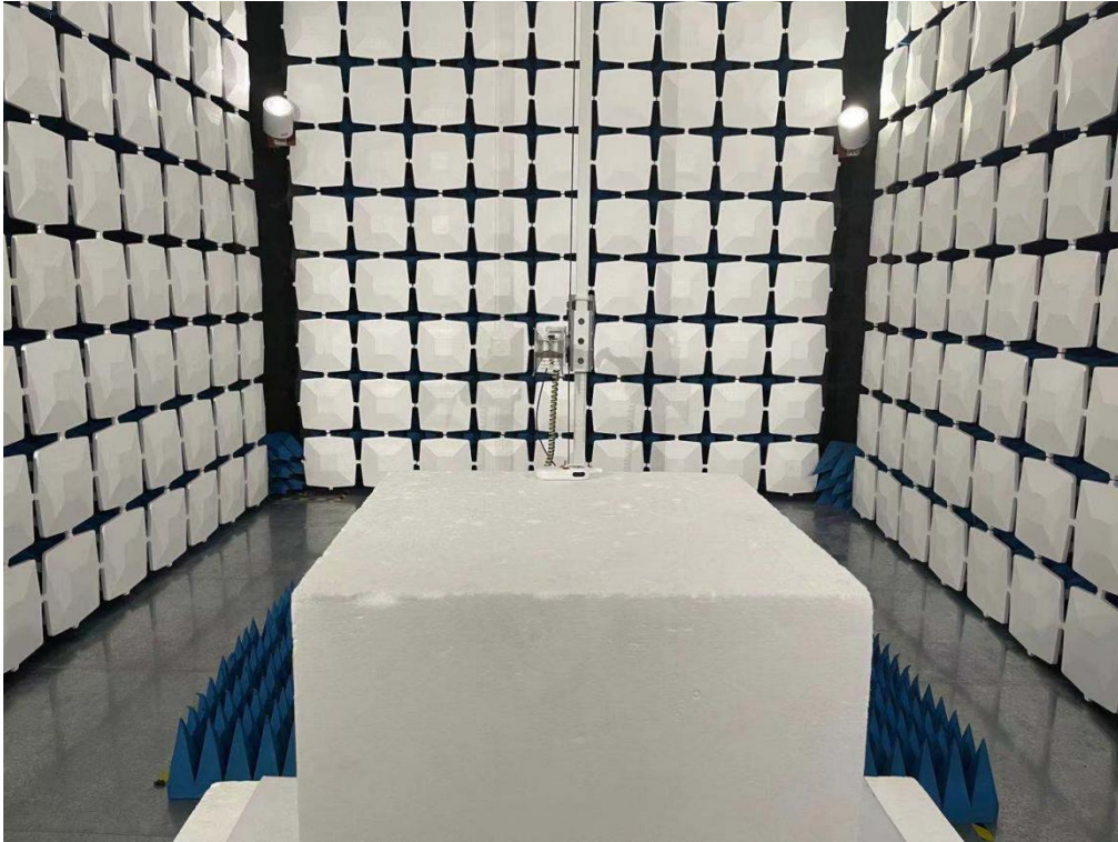
Above 1GHz for radiated emission test setup
