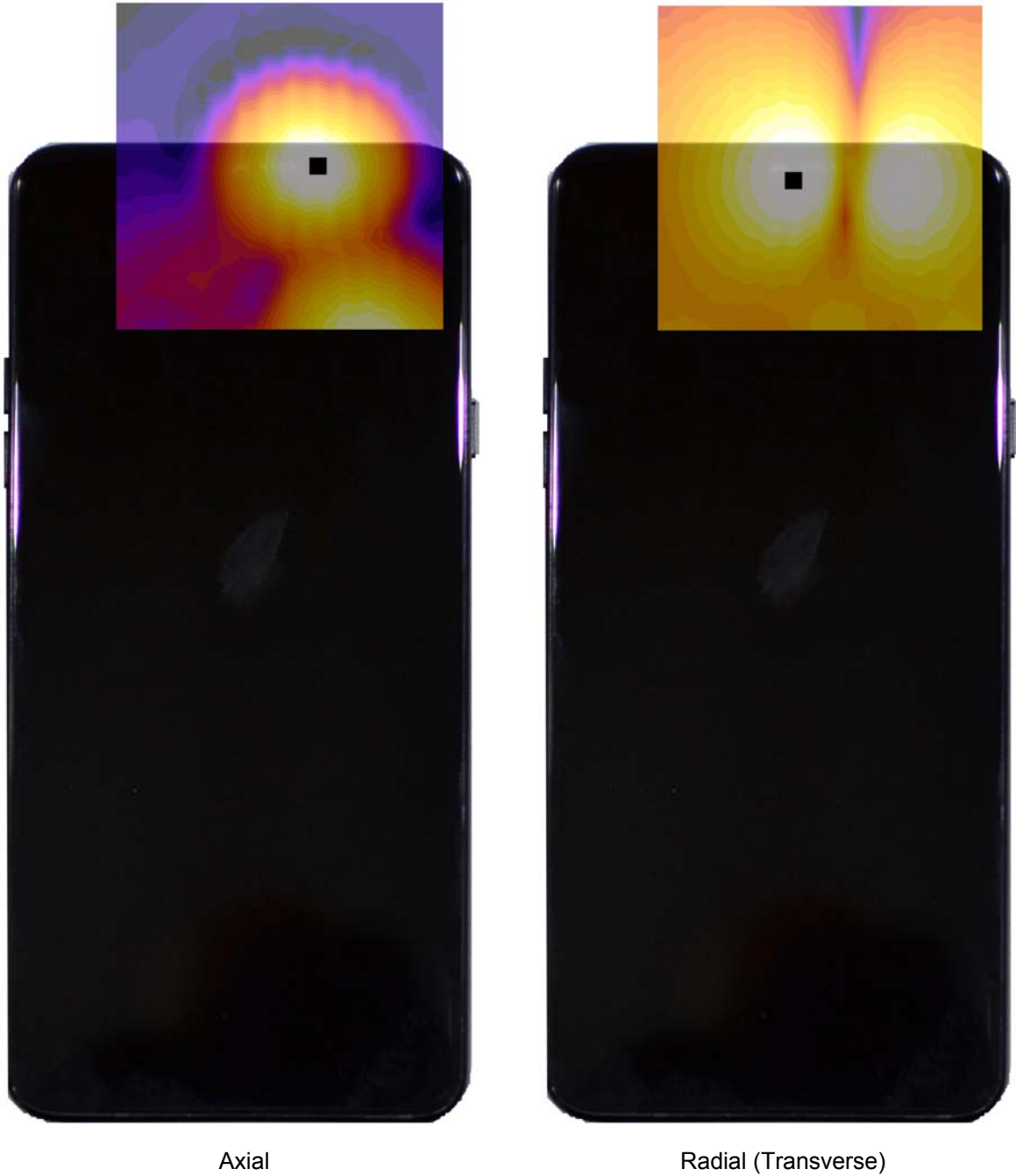
Figure 16-3 T-Coil Scan Overlay Magnetic Field Distributions
