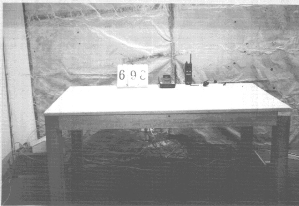
Fig. 2 Conducted Emissions Test Configuration (Operating only)
